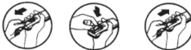
1. Slide open the cover according to the direction indicated by arrowhead.
